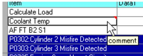
**Fig. 5-3-3: Tool Chip Display of Memo Contents**
